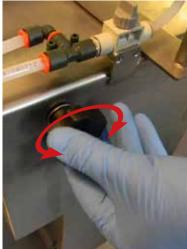
Connect the water feeder to the meat ball rounder and fasten securely with the black plastic knob.
