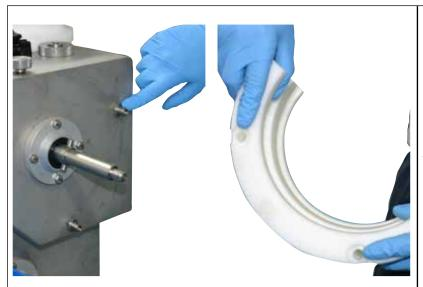
Replace the white arc, locating the holes onto the two studs of the machine.
