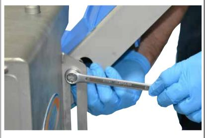
Maximum inclination. Tighten the screw again
