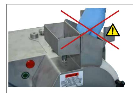
Do Not EVER insert your hands inside the hopper. DANGER OF CRUSHING Press the RED STOP button for the machine to stop
