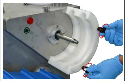
Loosen the two knobs on the white arc by turning them anticlockwise
