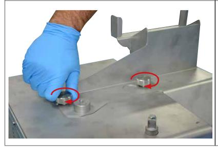
Once positioned correctly tighten the two securing screws.
