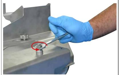
Using a 13 mm spanner, turn the nut anticlockwise to raise the height of the meatball rounder.
