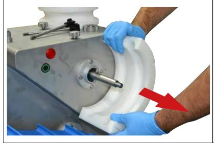
Remove the arc by pulling carefully towards you. Wash and carry out maintenance necessary and then proceed to reinstallation of the rounder.
