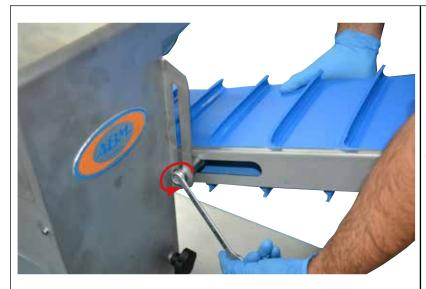
Using a 13 mm spanner, loosen the nut by turning it anticlockwise.
