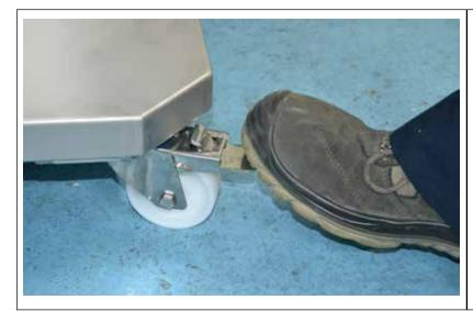
Wheel the machine into the production area and lock the machine into position, using the 2 braked wheels.
