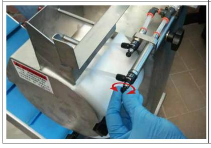
You can regulate the flow of water by adjusting the black regulators near to where the water exits the two white tubes. When the meat ball rounder is stopped it is advisable to turn the water off with the main tap. The water feeder is necessary mainly for a very sticky product to allow easy rolling through the rounding rollers. If for instance it is a meat product with little additives added it may work well without the water feeder.
