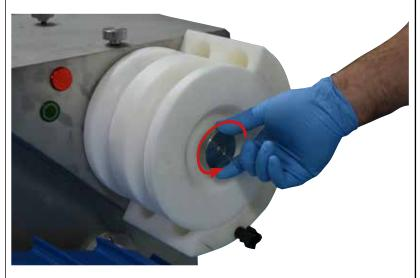
Unscrew the rounder locking nut by turning it anticlockwise
